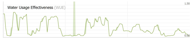
Figure 1. Direct WUE of Facebook's data center in Prineville, OR (Feb. 27 to May 28, 2013) [6].
